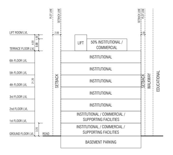
\* The minimum height between the finished ground floor level and first floor level should be 3.2 meters.
